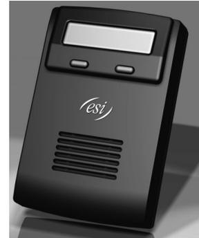
The ESI Presence Management application consists of just a few components. The RFID Reader is a wall-mounted RFID device containing components required for "tag and track" applications. The Reader's RFID transmitter is the electronic key device. This element can be in the form of a scan card or a keychain-type fob.
